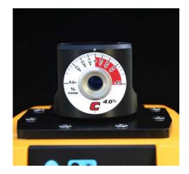
The standard cone scale provide a cone angle of  $\pm 4.0\%$ . There is an optional cone rotor that has a higher resolution scale and provides a cone angle of  $\pm .17\%$ .
