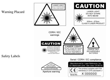
Note: The Alpha C is a CDRH class II laser and an IEC 60825 class 2 laser. It conforms to applicable EC directives regarding RFI and EMI, and to FDA performance standards 21 CFR subchapter J.
