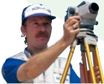
The SDL30 digital level makes accurate distance measuring easy. Simply aim at the unique RAB-Code staff, adjust the focus and press a single button to accurately measure height and distance. The results are shown on the LCD display and recorded in the internal memory – making the SDL30 the ideal instrument for quick and easy leveling.
