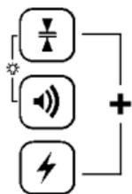
**Zero Deadband** – Super fine accuracy (0.1mm) used when calibrating lasers.
