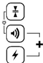
**Line Alert** – Special application to signal when the detector moves off on-grade.
