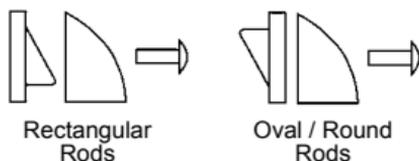
The slanted face grips tightly to round and oval rods. The flat face grips tightly to rectangular rods. To change the face of the jaw, remove the screw with a flathead screwdriver, flip the face over, and secure the screw back into the face.
