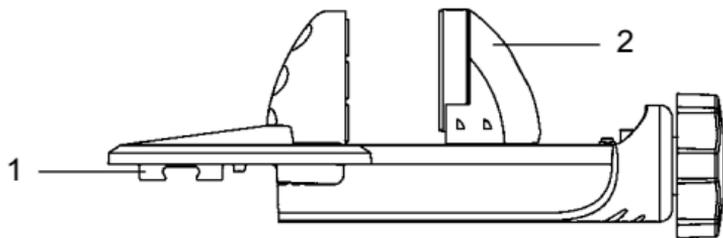
1. Dovetail slots - attaches clamp to the back of detector.
