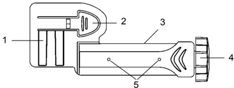
1. Dovetail slots - attaches clamp to the back of detector.
