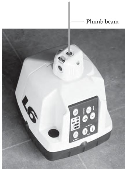
The L6 is designed for easily transferring points from floor to ceiling. As shown in the photo at left, once a point is established, simply draw intersecting lines through the point at 90° for a reference. The L6 has a notched base that allows you to quickly position the laser on this intersection, centering it over the point.
