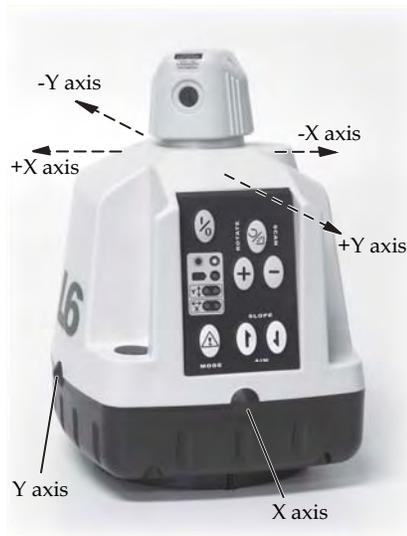
3. Return to the laser and turn the entire laser 180 degrees. The opposite Y-axis direction should now be aimed at the target. Allow the laser to re-level and mark the laser beam on the target.
