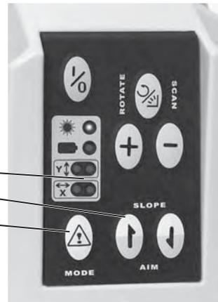
The RC-1 remote can be a valuable addition to your system. It provides all of the normal adjustments on the laser control panel and allows you to make these settings from up to 100ft. (30m) away when working indoors. Especially when the laser is set-up out of normal reach, the remote provides a quick and convenient way to change the laser's settings.
