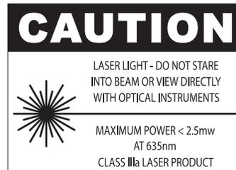
The L6 transmitter is a class IIIa (less than 2.5mW) laser under the United States C.D.R.H. guidelines.
