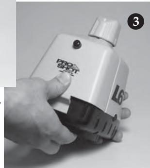
Hook battery door at top of housing and push firmly at base of door to latch
