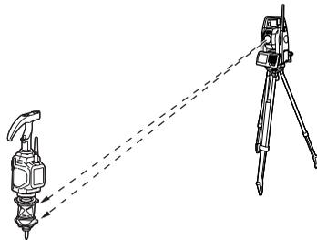
5. The SX/NET tracks a sighted prism as it is moved to the next measurement point when Auto Tracking is set.
