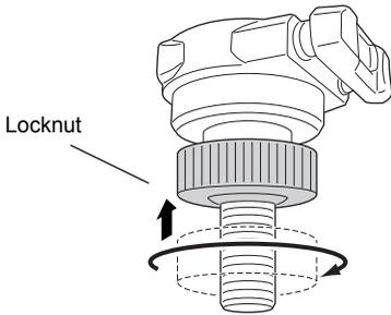
1. Rotate the locknut counterclockwise until it reaches the upper limit.
