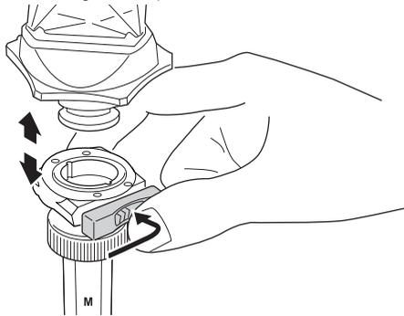
● **Attaching the One-touch attachment (SB179A) to the range pole (AP67/67A)**
