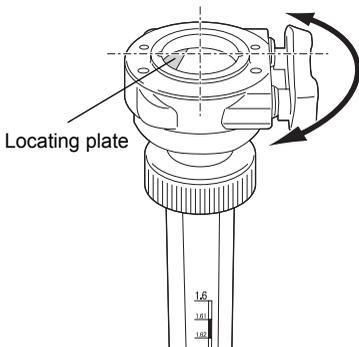
3. Adjust until the locating plate is on the left (with the graduations facing forward).
