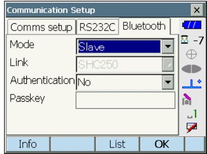
3. The display returns to Meas mode and SX/NET enters "Waiting" mode. The Remote Controller searches for the total station wireless device and initiates a connection.
