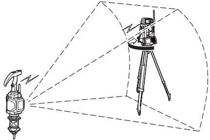
3. Once the position of the horizontal direction has been determined, the total station telescope then begins to rotate along the vertical axis searching for the position of the prism.
