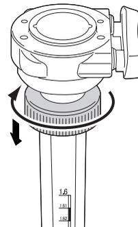
4. Rotate the locknut towards the pole until secured in place.
