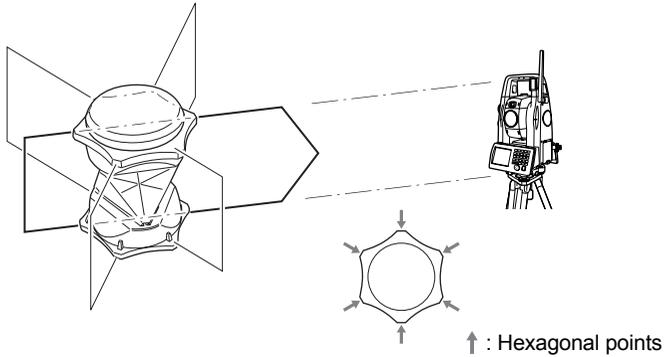
When using the ATP1S, the 360° Prism should be set up so that a pair of diametrically-opposed marks on top of the prism are aligned with the sighting direction of the total station.
