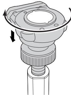
2. Rotate the One-touch attachment clockwise until the locknut meets the top of the pole.
