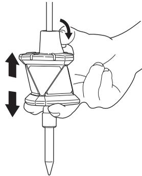
● **Connecting the 360° Prism to the Remote Controller**
