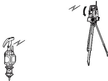
4. Once the position of the vertical direction has been determined an audio sounds and the total station automatically sights the prism in the field of view.
