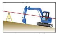
In combination with Topcon's rotating slope lasers, you will get excavate with the right slope.
